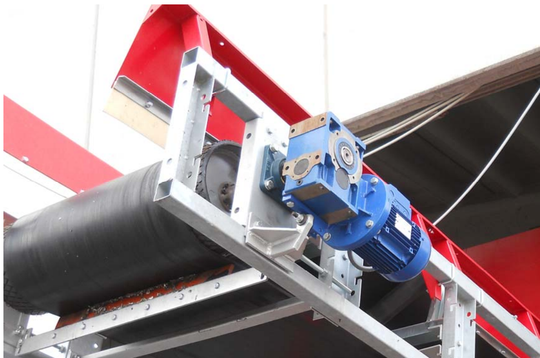
Figure 11 Gear motor and bearing support of drive roller
